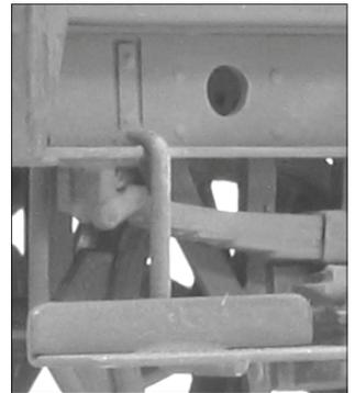
Fit end window rainstrips (parts 10) wide ones to the top and narrow to bottom. Form up the lamp irons (parts 11) and reinforce the folds with 60/40 solder. Fit the lamp irons to the body sides and ends noting that there are etched marks to help with positioning.
